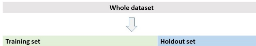
Figure 8: The holdout method. The whole dataset is split into two parts: training and holdout sets.
